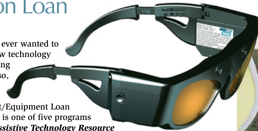
iGlasses— a head-mounted device that uses ultrasonic sensors.
